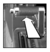
While still pressing the button, move the lever forward as far as it will go. Let go of the button and the lever.
